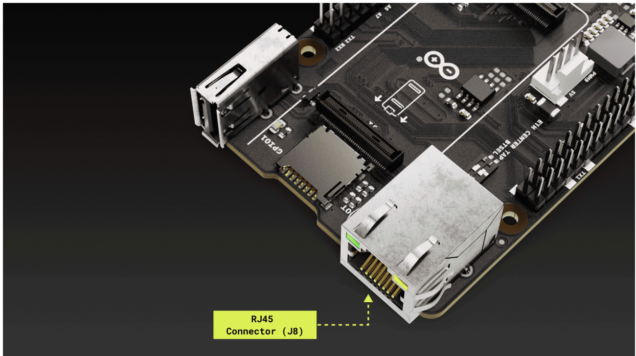
Figure 11. RJ45 connector of the Portenta Hat Carrier
